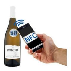
NFC is a wireless technology that's embedded into most smartphones. It has an array of applications from mobile payments to NFC tags embedded into products, labels and promotional material. The beauty of these tags is that they interact with consumers' smartphones using a radio signal. And, unlike Bluetooth, you don't have to manually pair two NFC devices. They also use a fraction of the battery power used by Bluetooth and Wi-Fi.
