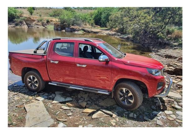
The vehicle can be fitted with 1 to 4 cameras to facilitate manoeuvring both in town and on the road. The off-road camera (in the passenger rear-view mirror) and 360° vision support the driver when negotiating obstacles or narrow trails. In addition, they can be set to automatically activate when obstacles are detected.
