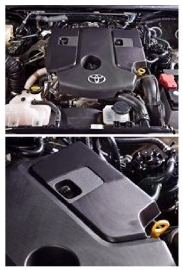
The focal point of the new "mid-range" 2.4 litre Global Diesel (GD) engines are undoubtedly their impressive power and torque outputs. The new engine bows in to replace the previously employed 2.5 litre D-4D, and brings with it a vast range of improvements in performance, refinement and fuel efficiency. Retaining the proven DOHC 16 valve, inline 4-cylinder architecture, the new engines bring with a number of advancements under the skin.
