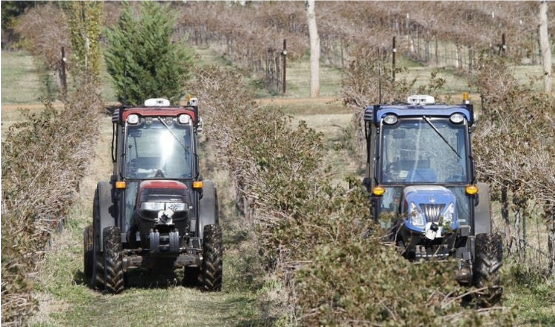
Two driverless tractors spray vines in a Texas vineyard. Each one is controlled from a single command station (2012).
